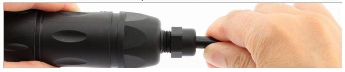
3. Screw the head nut using a 15 mm U-wrench. Tightened the head nut with a 2 Nm torque.
