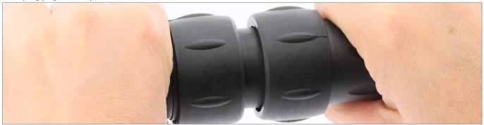
3. Slide the blackshell and screw it using a 28 mm U-wrench. Tightened the backshell with a 4 Nm torque.
