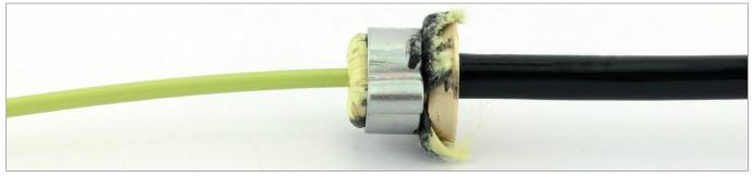
9. Crimp the both ear of the Clamp using the Nipper. Remove the kevlar strength members using using the shears.
