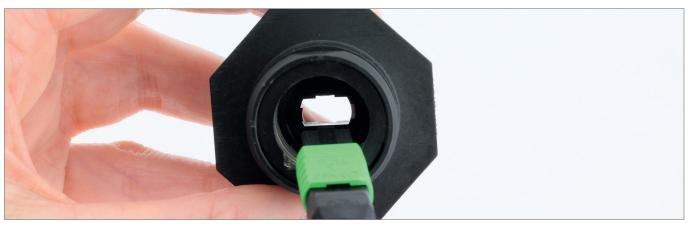
$4.\mbox{Seat}$  o-ring, place receptacle in the panel cut-out.
